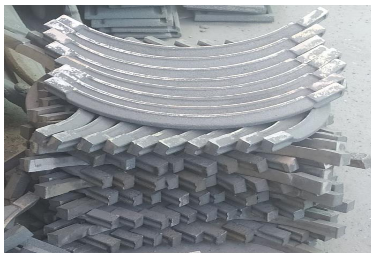
Fig.-7 Ready Rib by Steel mold with
