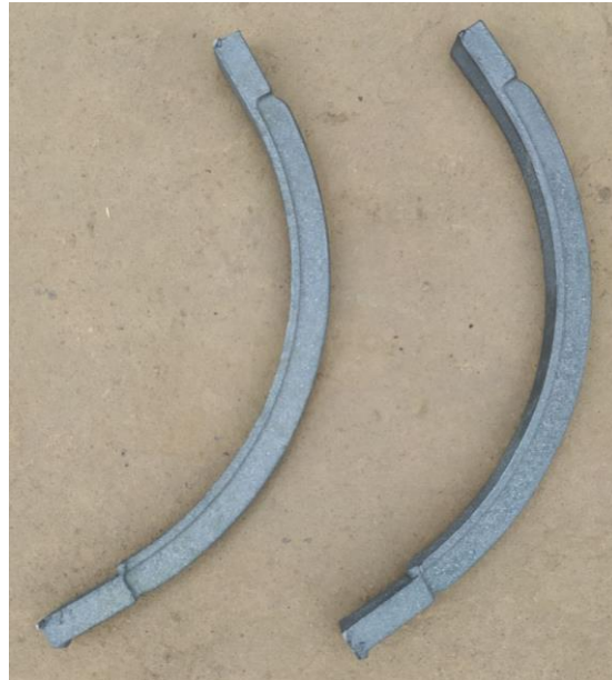
Fig.-5 Ready Rib by Aluminiiy mould
