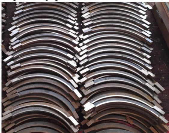
Fig.-3 Ready Rib by MDF mould
