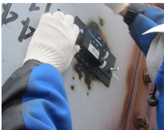
Figure 1. Mobile bridge monitoring system
