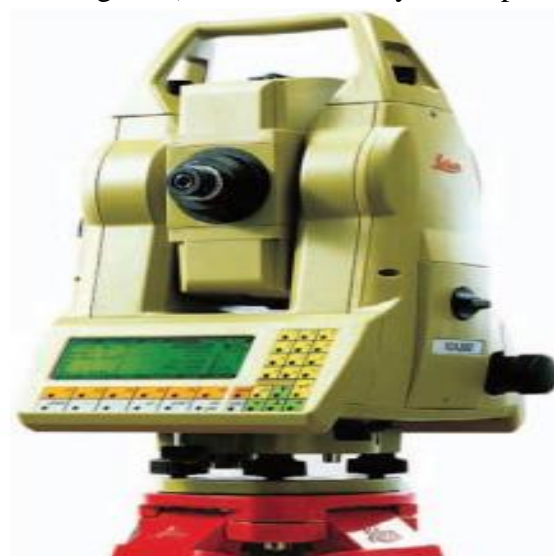
Figure 1: TCA2300 universal total station.( equipment for calculating the accuracy of the slope angle).
