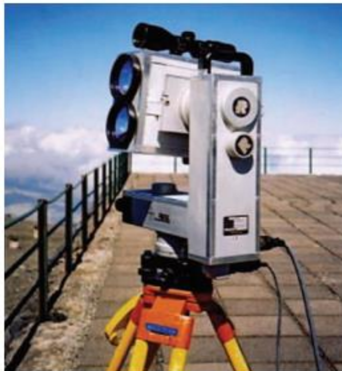
Figure 2: Laser scanning unit (LPM-2K Determining the dimensions of the mining slope by laser beams)
