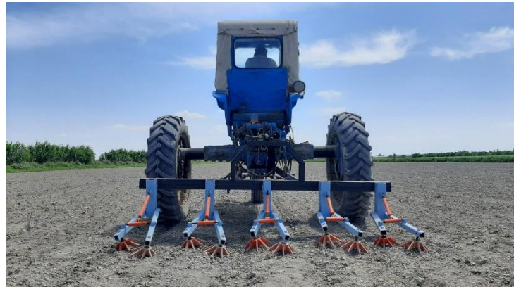
Figure 5. Procedure for pilot testing of the proposed cotton softening device.
