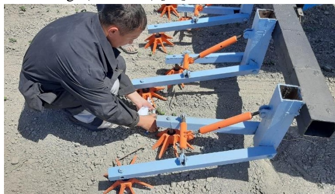
Figure 4. The process of matching the recommended fluff softening device to the cotton row spacing.
